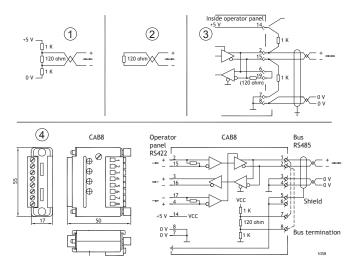
Some (older) operator panels had pull-up and pull-down resistance except for the actual bus termination at  $120 \Omega$ , similar to Westermo and Profibus. See 1 in drawing above.
